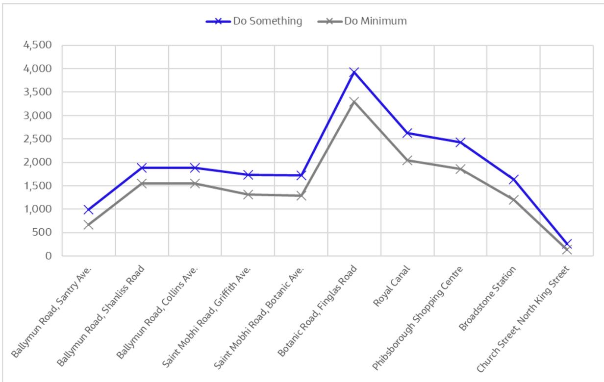
**Image 2.9: 2028 AM Peak Hour Passenger Volume Along Proposed Scheme (Inbound Direction – Ballymun Section)**
