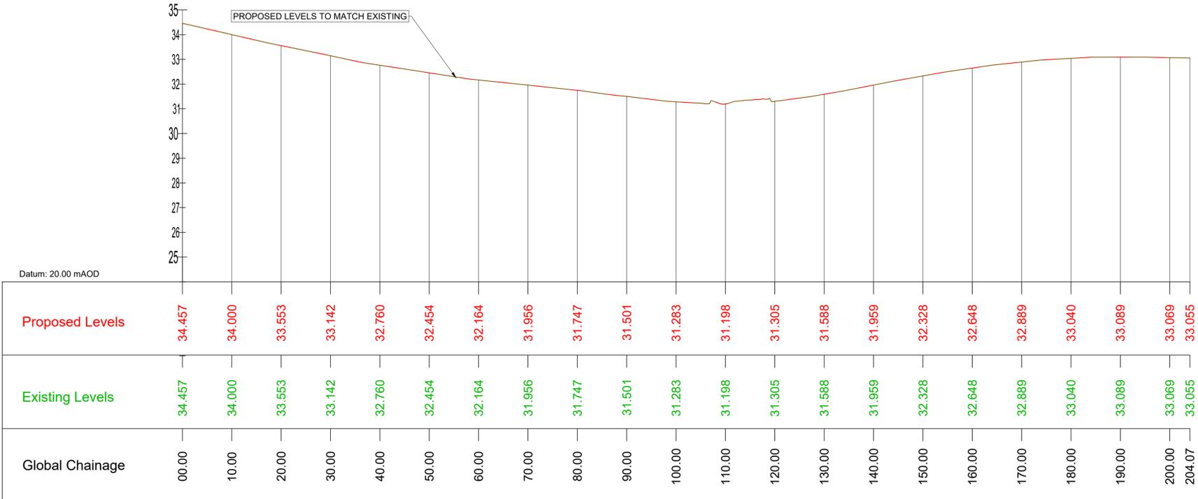
GEO\_HV-0304\_SR\_01-M3-CR-0001-C01 LONGITUDINAL SECTION
