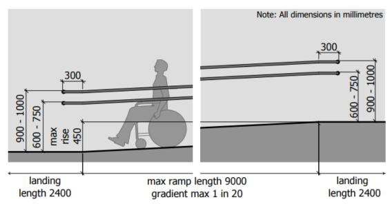
Figure 25. Examples of external ramp
