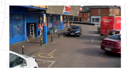
ON STREET-ACCESSIBLE CAR PARKING. DIMENSIONS AND SIGNALS MARKS TO BE REVIEWD. DIMENSIONS OF 3.6 x 7 m. AS PER TGD-M.
