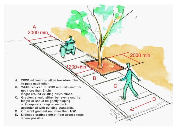
Figure 5. Urban environment pavement layout
