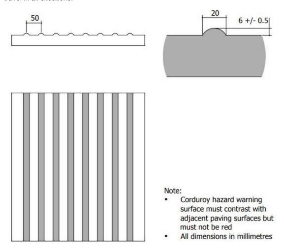
Figure 21. Corduroy tactile paving tile and raised bars dimensions.
