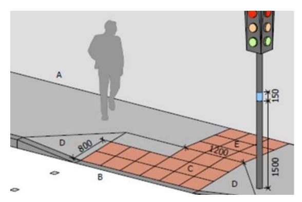
Figure 17. Controlled Crossing. Not in Direct Line of Travel
