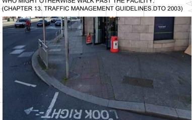
DETERIORATING PAVEMENT IN UNCONTROLLED CROSSING POINT? DISHED KERB TO BE PROVIDED AND "BUFF" OR GREY TACTILE PAVING.
