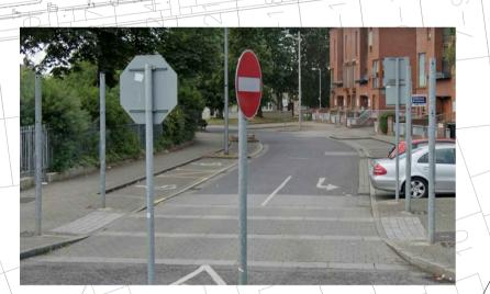
UNCONTROLLED CROSSING POINT. BUFF OR GREY TACTILE PAVING SHOULD BE PROVIDED: 3 SLABS.
