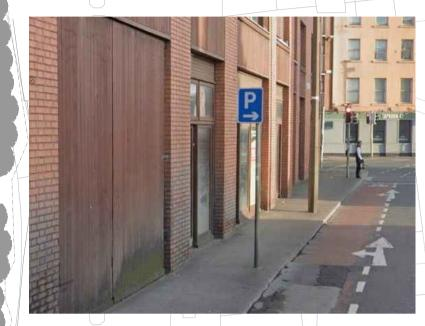
AN ALTERNATIVE LOCATION OF THE SIGNAL POLE SHOULD BE CONSIDERED. REDUCED WIDTH OH FOOTPATH < 1.20m.
