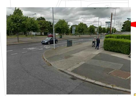
PROVIDE BUFF OR GREY TACTILE PAVING. 1200mm. FOR UNCONTROLLED CROSSING AND DISHED KERB.
