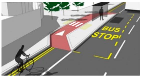
Example of a bus stop bypass solution
