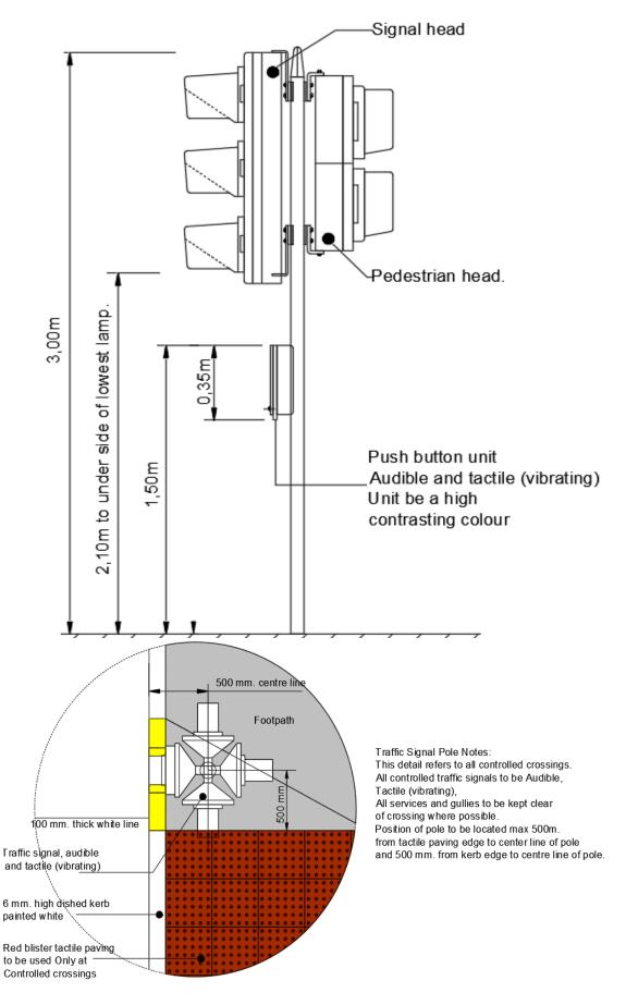
Figure 23. Plan and Elevation of traffic Signal
