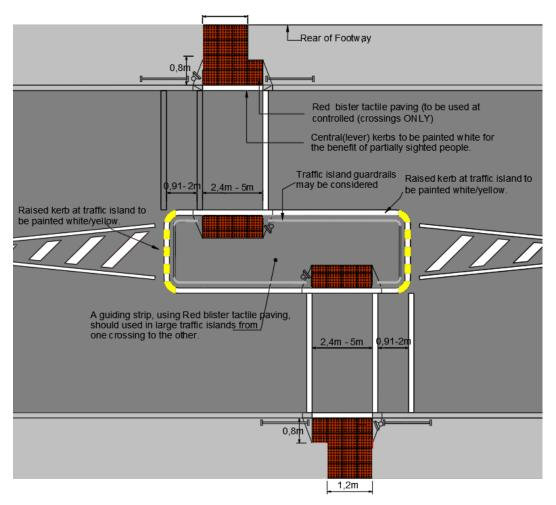
Figure 18. Controlled Crossing. Staggered Signalized Crossing
