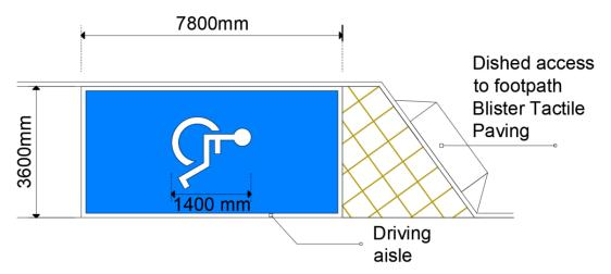
Figure 3. Example of Parallel parking
