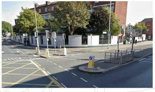
IN THE DESIGN PROPOSED, THE FOOTPATH IN THE CORNER BECOMES WIDER. STAGGERED CROSSINGS POINT IS RECOMMENDED WHEN POSSIBLE TO BE REMOVED. A DIRECT CROSSING SHOULD BE COMFORTABLE AND AVOID PEOPLE TO GET STUCK. FOLLOW MEASURES OF ACCESSIBILITY FOR THE NEW CROSSING PROPOSED. (RED BLISTER TACTILE PAVING, DISHED KERBS, AUDIBLE SIGNALS, ETC.)
