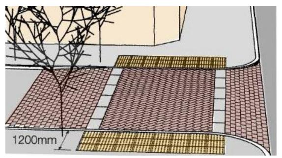
Layout of blister tactile paving at a side road junction where the side road carriageway has been raised to the level of a footway.
