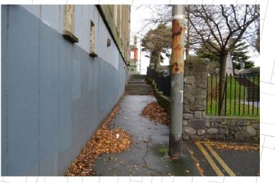
CHANGE IN LEVEL. NO ACCESSIBLE PASS. A NEW UNDERPASS FOR CYCLE ROUTE AND PEDESTRIANS IS PROPOSED. TACTILE WARNING SURFACE (400MM.MIN) AT THE START/END OF THE STAIR SHOULD BE CONSIDERED AND A CONTINUOUS HANDRAIL ON EACH SIDE OF FLIGHTS. AN ALTERNATIVE ROUTE
