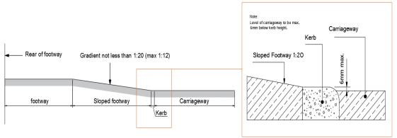
Figure 8. Dished Kerb Section Detail
