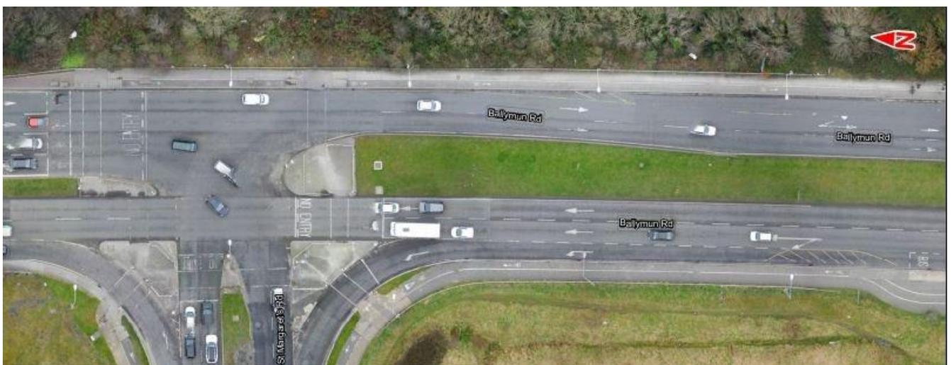
**Image 5.1: R108 Ballymun Road / St Margaret's Road Three-Arm Signalised Junction**
