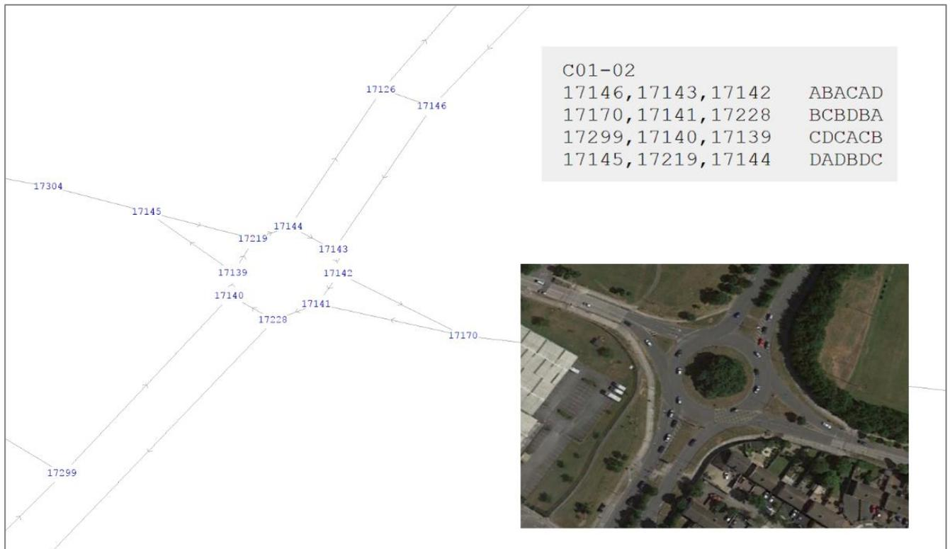
**Diagram 4.3: Bus Connects LAM Node Matching (Junction C01-02)**
