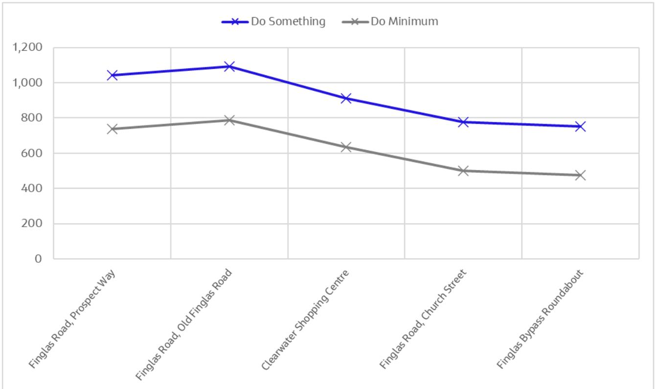
**Diagram 6.15: 2043 PM Peak Hour Passenger Volume Along Proposed Scheme (outbound direction – Finglas to Phibsborough)**
