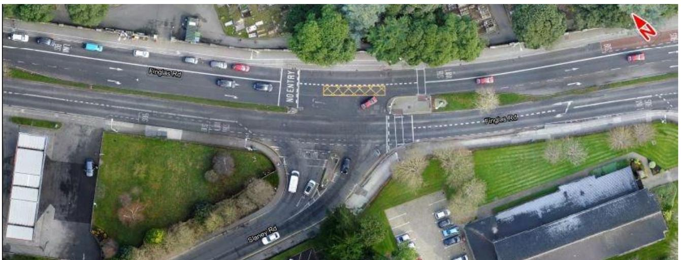
**Image 5.30: R135 Finglas Road / Slaney Road Three-Arm Signalised Junction**
