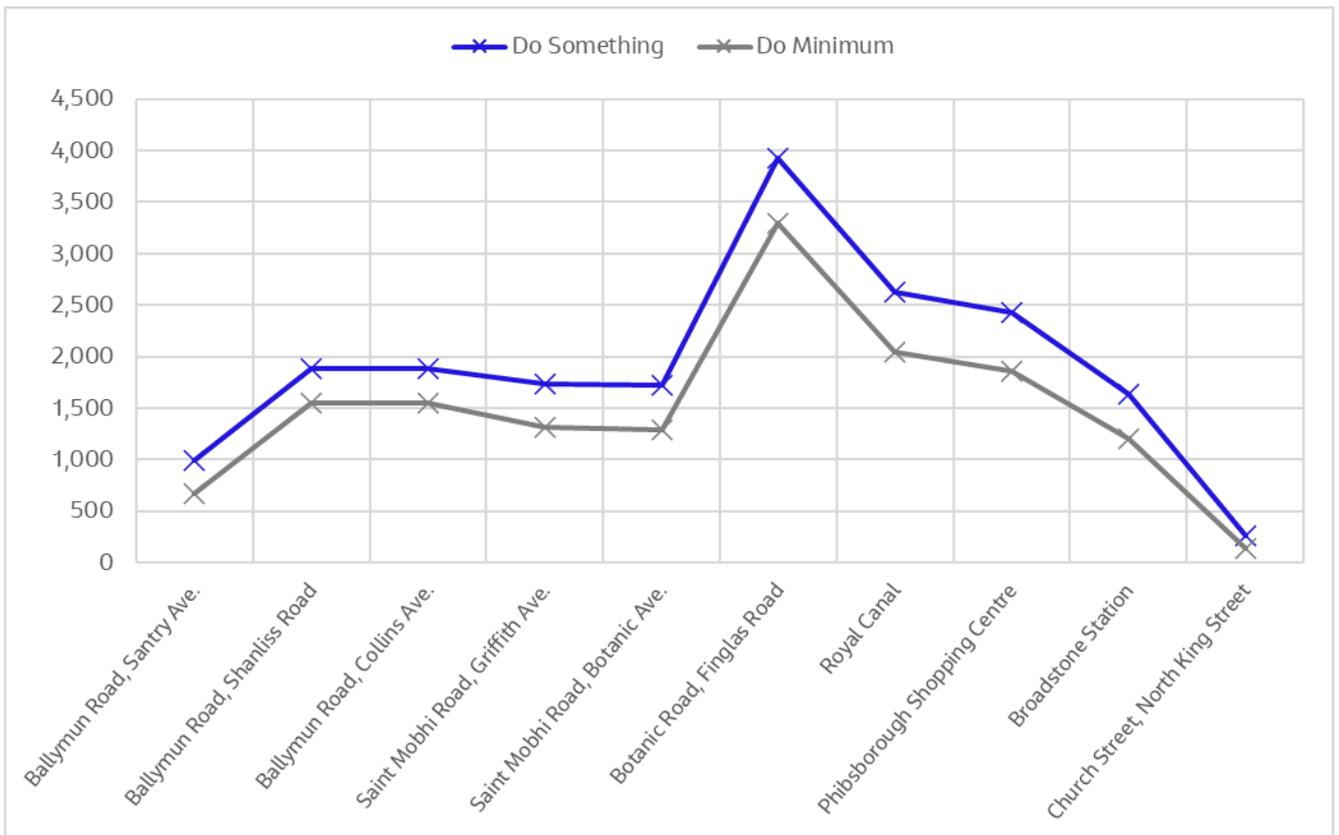
**Diagram 6.8: 2028 AM Peak Hour Passenger Volume Along Proposed Scheme (inbound direction – Finglas to Phibsborough)**
