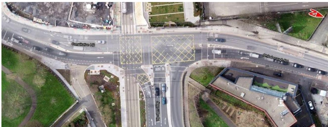
**Image 5.17: R108 and R135 Phibsborough Road / R135 Western Way / R108 Constitution Hill Three-Arm Signalised Junction**
