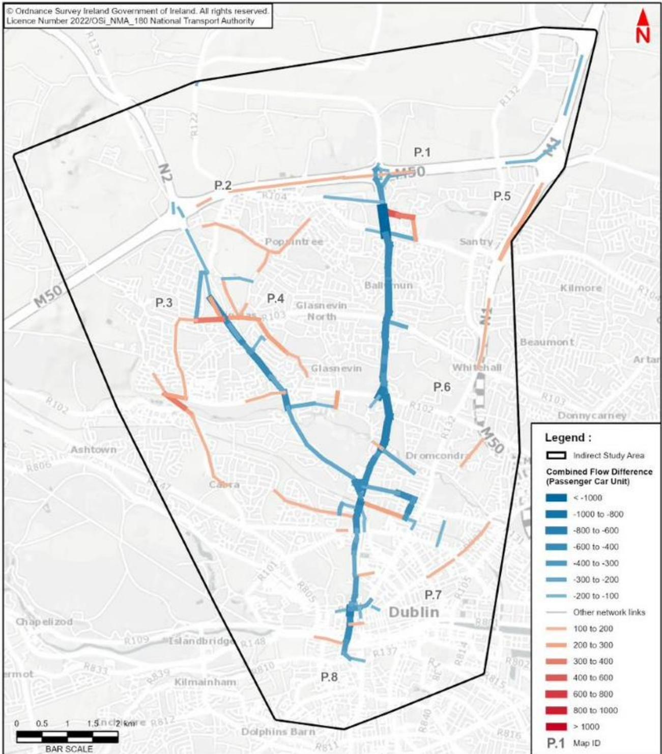
Diagram 6.39: Flow Difference on Road Links (Do Minimum vs Do Something), PM Peak Hour, Opening Year (2028) Impact on Direct Study Area (PM Peak Hour)
