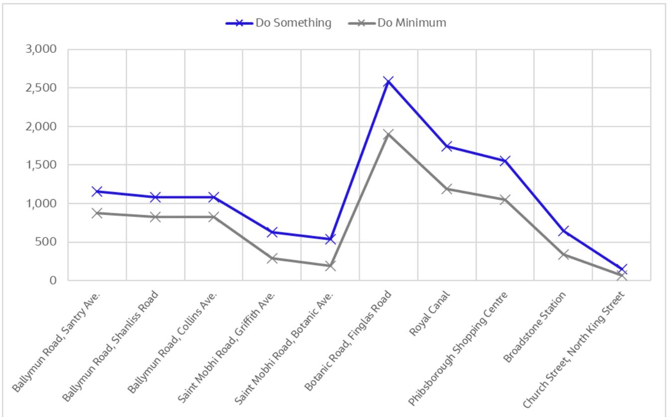
**Diagram 6.12: 2043 AM Peak Hour Passenger Volume Along Proposed Scheme (inbound direction – Ballymun to City Centre)**
