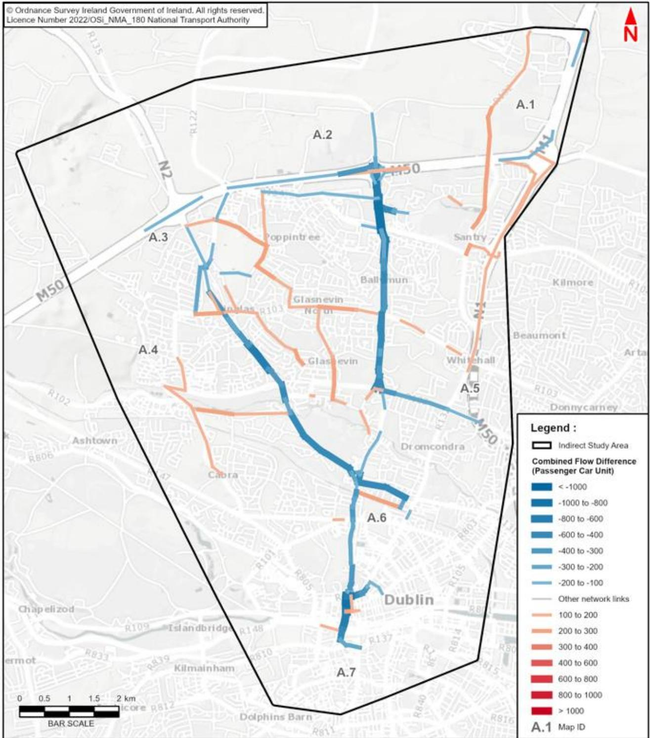
**Diagram 6.38: Flow Difference on Road Links (Do Minimum vs. Do Something), AM Peak Hour, Opening Year (2028)**
