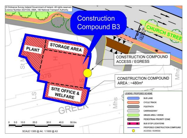
Image 7.3: Location and Extent of Construction Compound B3
