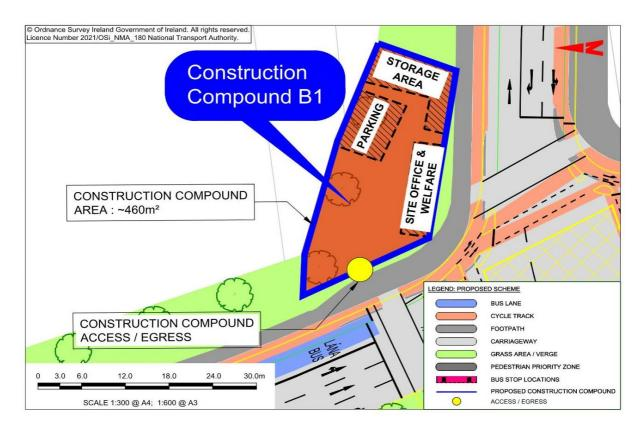
Image 7.1: Location and Extent of Construction Compound B1
